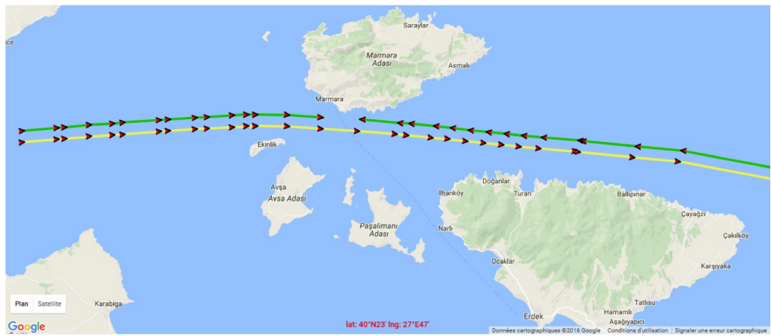
Figure 15: AIS data manipulation to simulate a collision between a fishing vessel and a Cargo vessel
